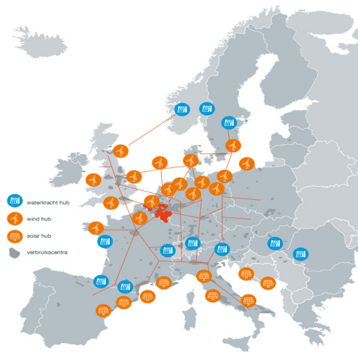
Graph 5 Simplified representation of load centers (dark grey), wind and solar (orange) and water (blue) in Europe
